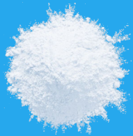
Polygloss 90 Speciality KAOLIN TiO_2 substitute for Solvent/ water based paints & inks KaMin (USA)
